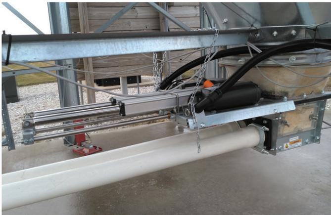
Single or twin options are available. Automatic opening based on load cell, or proximity switch inputs.
